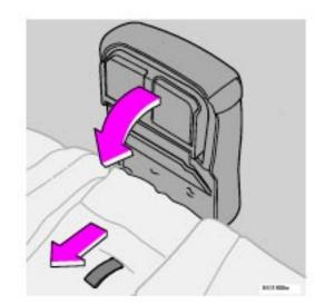
To close: Fold the table section upward into place. Fold the arm under the table inward being careful not to pinch your hand. Pull the release and fold the table section back in place.
